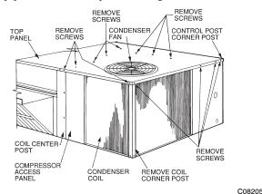
Fig. 8 - Cleaning Condenser Coil
